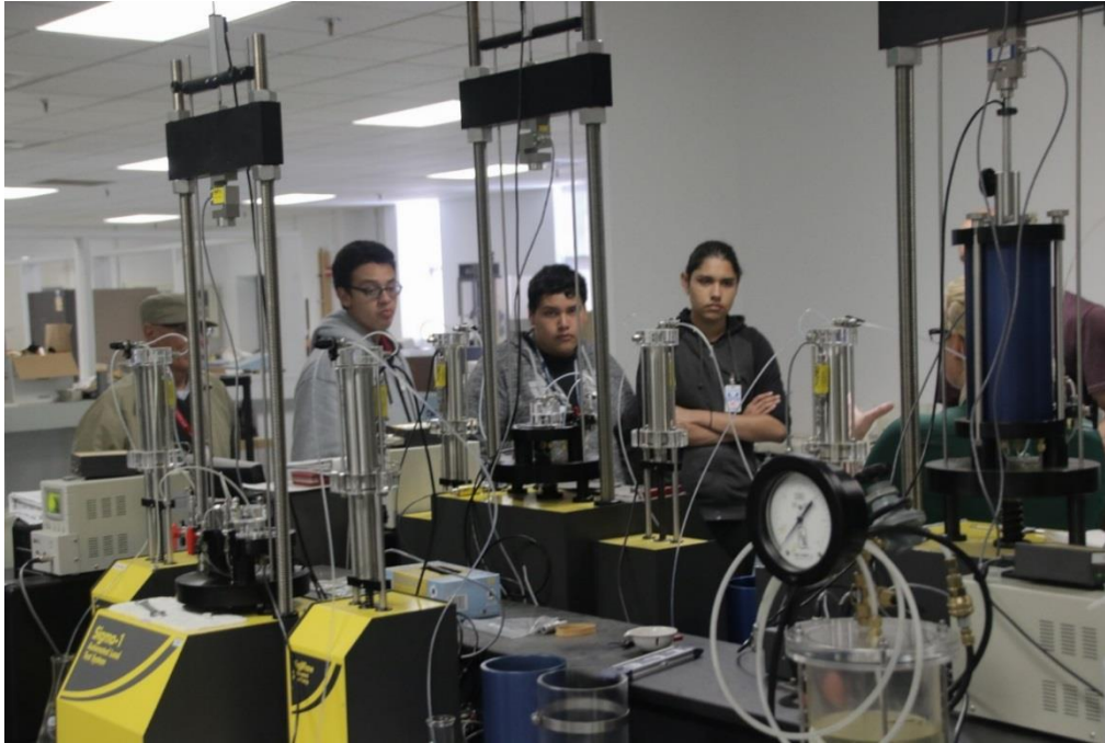
Triaxial equipment to determine shear strength of a soil
